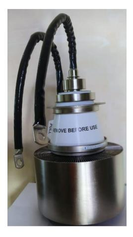
Pilani Electron Tubes & Devices Pvt. Ltd. Patiala Road, Sangrur, PB, 148001, India Phone: +91-9815309603 Email: sales@pilanielectron.com Website: www.pilanielectron.com PET1647F is a power triode of coaxial ceramic-metal construction. It is intended primarily for industrial RF heating machines. Anode is cooled by forced-air.
